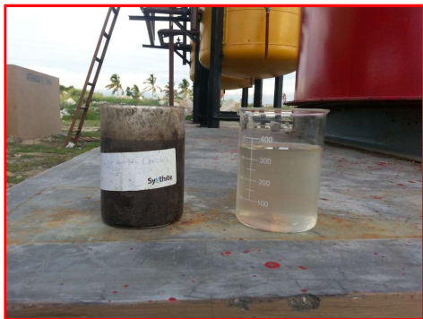
RAW & TREATED EFFLUENT SAMPLES Location : Site
